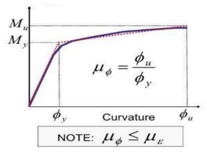
Moment curvature in Inelastic Behavior to Section
