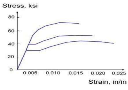
Stress-Strain curve for Steel
