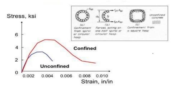
Stress-Strain curve for Concrete (Unconfined and Confined)
