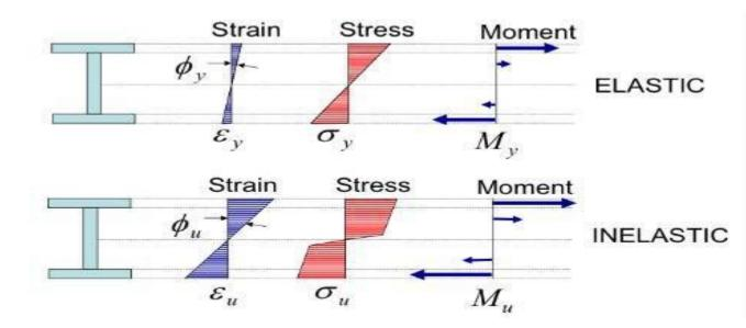
Elastic and Inelastic Behavior in Section
